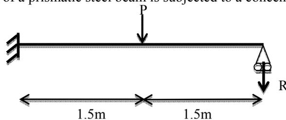
Q.48 If load  $P = 80 \text{ kN}$ , find the reaction  $R$  (in  $\text{kN}$ ) (correct to 1-decimal place) using elastic analysis.
